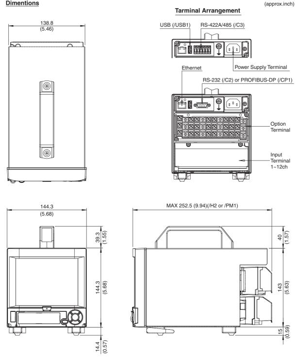
If not specified, the tolerance is  $\pm$ 3%. However, for dimentions less than 10mm, the tolerance is  $\pm$ 0.3mm.
