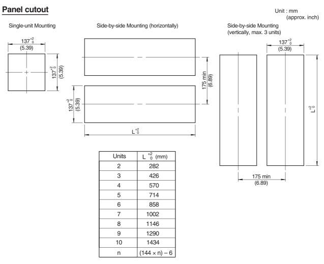
Note : If not specified, the tolerance is ±3%. However, for dimensions less than 10 mm, the tolerance is ±0.3 mm.
